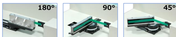
Figure 1 – Sample stage in different positions
