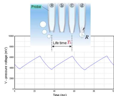
Using the Laplace equation, the bubble pressure method measures the maximum pressure and determines the surface tension.
